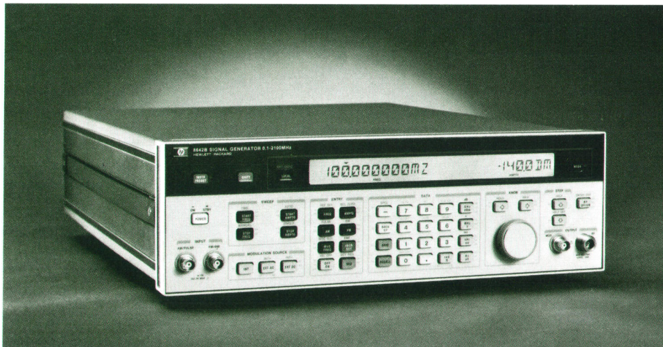
Fig. 1. The HP 8642A/B Signal Generator uses new low-noise oscillator designs with high-Q surface-acoustic-wave (SAW) resonators to improve spectral purity over cavity-tuned generators. Its frequency range is 100 \text{ kHz} to 1057.5 \text{ MHz} (A model) or 2115 \text{ MHz} (B model). High accuracy, wide output power range, and broad modulation capabilities make it suitable for the most stringent receiver tests.
